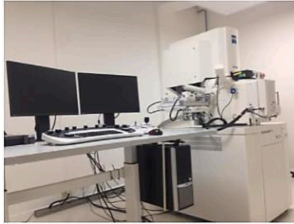
Fig. 6. Experimental Setup for Scanning Electron Microscopy (ZEISS brand).
