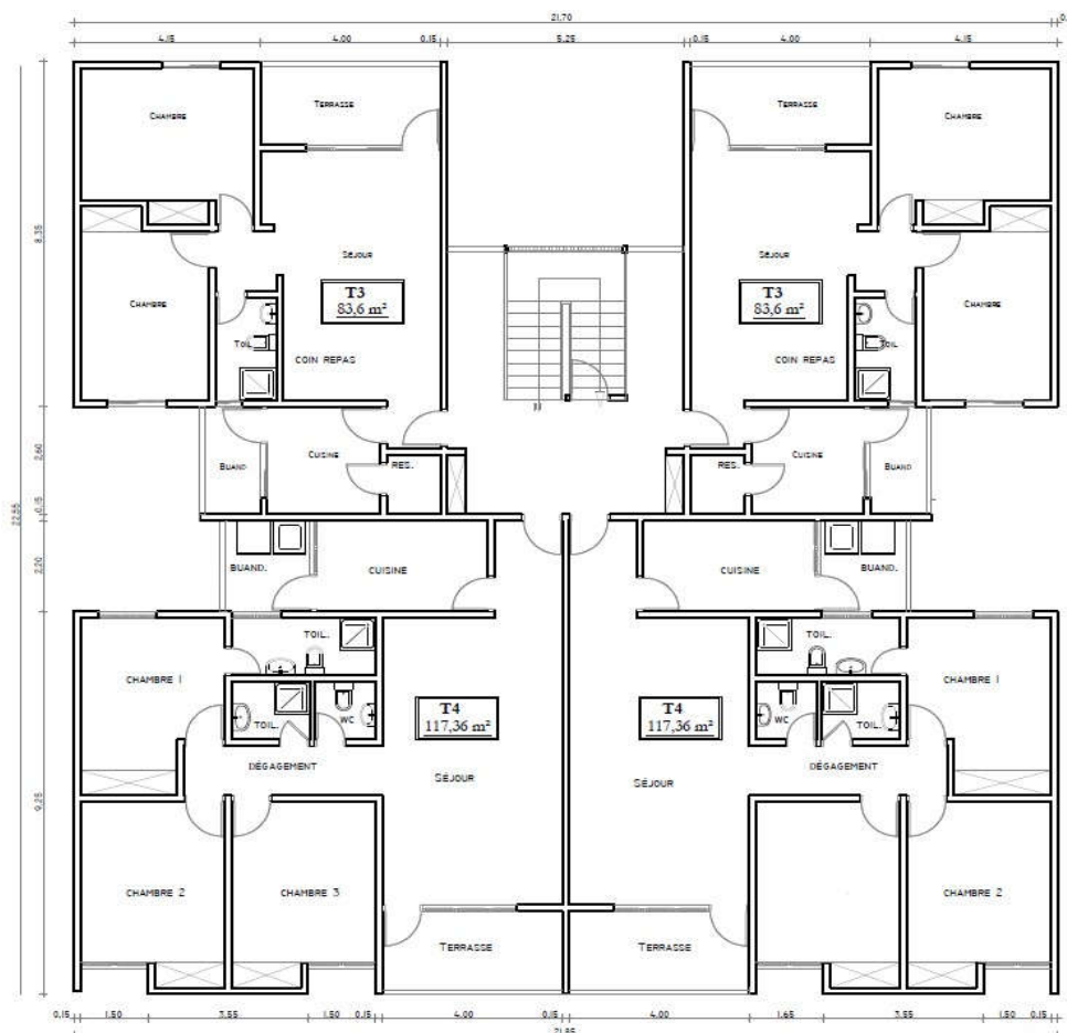
Figure 1. Plan of the standard storey of the model of the building under consideration
