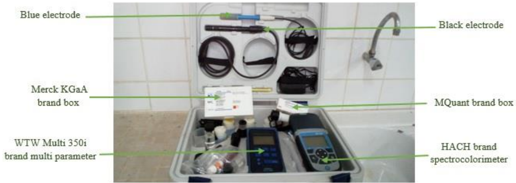
Fig. 1: kit instruments of the analysis equipment used
